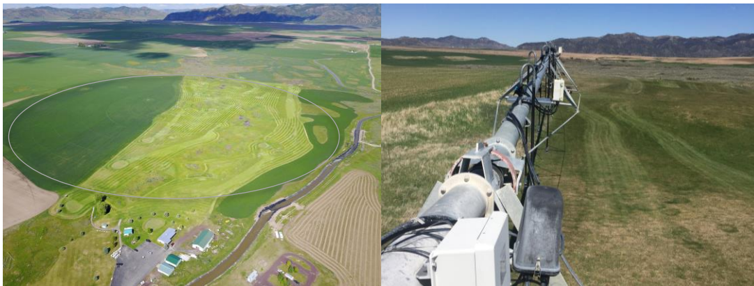
The pilot study will be conducted at Christensen Farms in Grace, ID. The left image shows the center-pivot sprinkler that waters both a crop field and a golf course. The right image shows GPS receivers, controllers, and nozzles on the existing variable rate irrigation system.
