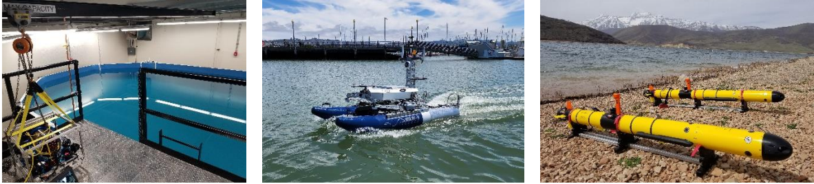
Figure 3 – Our 20ft x 30ft x 6ft AUV test tank, 1x Marine Advanced Robotics WAM-V ASV, and 2x OceanServer IVER3 AUVs.
